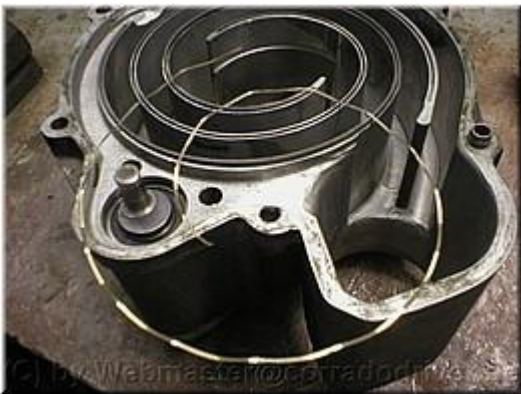
time to install springs (if you have them) and later - long apex strips inside the halves
