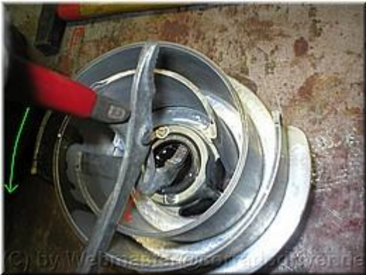
Sometimes somebody makes performance modification during G rebuild. If you rebore and polish these channels, more air will fly through supercharger and you will gain more horsepower finally. It's difficult modification. Often named 'RS modification'.
