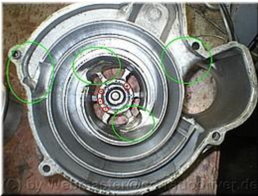
Sometimes somebody makes performance modification during G rebuild. If you rebore and polish these channels, more air will fly through supercharger and you will gain more horsepower finally. It's difficult modification. Often named 'RS modification'.
