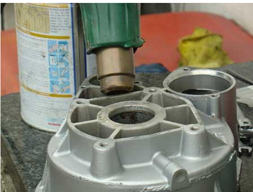
The best way to install bearings is simple. Preheat the bearing seat well (using for example heating gun) and don't forget put your bearing to the freezer for 30 minutes before installation. Bearings can be installed with a press too, but if the bearings are out-of-alignment, damage is almost certain to occur to both the bearing and charger. The circlips are reinstalled to hold the bearings in place taking great care that they are aligned so as not to block the oil ways that feed the bearings with oil. The oil seals are pushed into place and care is taken to ensure that the external seal on the main shaft is not pressed flush with the casing as fitting them to sit flush will obstruct the oil way that feeds the bearing. Bearing shouldn't fit to the end, unless circlip, which holds bearing move that to not cover the oil hole.
